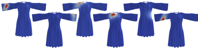
Fig. 4: Color plots of the first six approximated eigenvectors of the long-sleeved dress mesh, where vertices in red represent high values distributed in areas such as the sleeves, shoulders, waist, and neckline. This suggests that the spectral description can reveal meaningful global information of the mesh shape.
