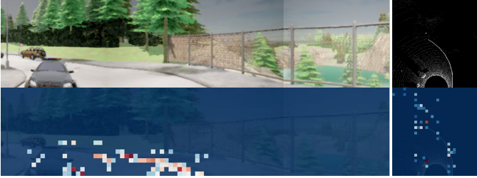
Fig. 16. Attribution results generated on the second feature level of TransFuser model. Given the model's multimodal input (image and LiDAR data), the attributions are correspondingly divided into two parts, reflecting the contributions of each modality.
